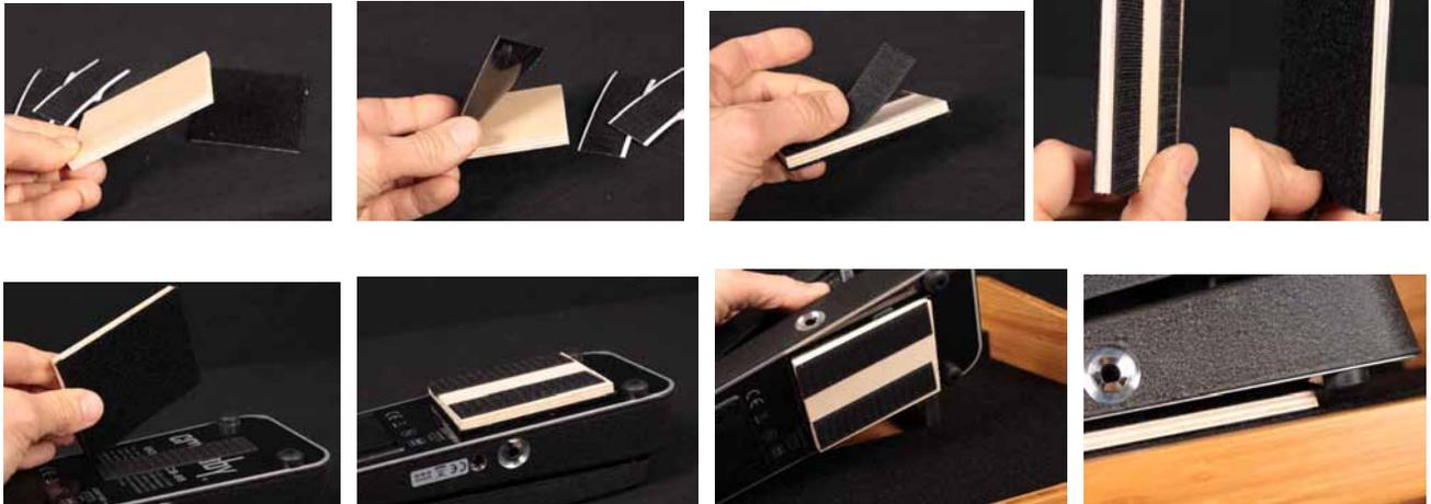
2. The hook & loop bond is stronger than you might think and as long as the adhesion issues are taken care of, you can usually get away with a lot less loop material than it takes to cover the bottom of the device. Obviously you don't want your pedals falling off the board, but the fact is that two non flexible surfaces bonded with industrial hook & loop are very difficult to get apart. So temper your use of the hook material based on how often you think you might be moving things around.
